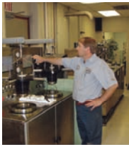
HT-HP "thickening time" testing is part of the Joppa Plant quality control process. Temperatures reach as high as 600° F.
